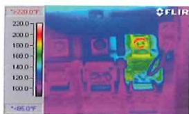
▼ Figure 4.5 Thermal image of contactor after loose termination has been tightened
