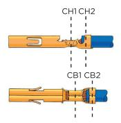
CH2: Insulation crimp height CH1: Conductor crimp height CB2m: Insulation crimp width CB1m: Condutor crimp width
