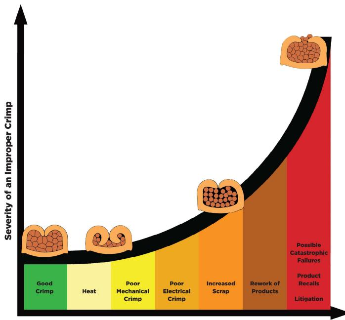
**Cost of an Improper Crimp**
