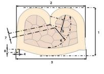
Dimensions of a conductor crimp
